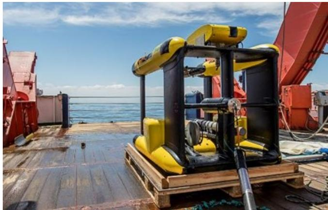
**Figure 2 (above).** The TRIAXUS, a towed remotely controlled underwater vehicle.
