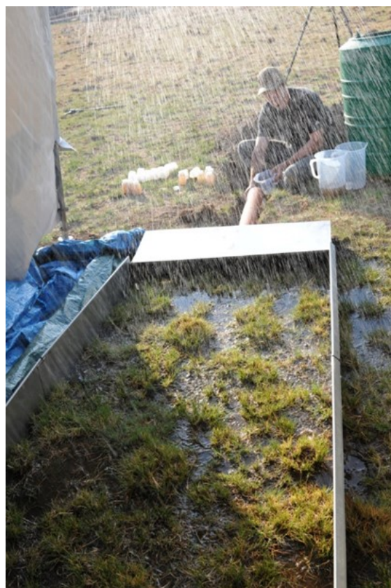
Figure 1 (left). Measuring runoff and sediment concentration at an experimental plot during a rainfall simulation experiment close to Ladybrand, Free State (Photo: J. Baade 2019).
