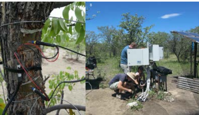
Fig. 3: Different sensor systems are installed in the field. Continuous sap flow measurements (A) are used to understand how water fluxes through woody plants are affected by different simulated browsing scenarios. Browsing is experimentally simulated by clipping leaves of single branches or whole trees at different ratios. Logger systems (B) store the continuous information alongside with additional data on climate, soil moisture, solar radiation and other environmental parameters are measured.
