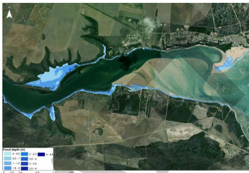
Fig. 2: Simulated compound flooding at the Breede estuary case study (from a compound event corresponding to the 1-in-100y river discharge, 1-in-100y waves and spring tide)
