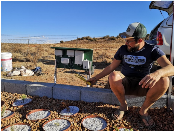
Fig. 1: Low-cost Arduino system that collects environmental data and sends it to the open-access cloud
